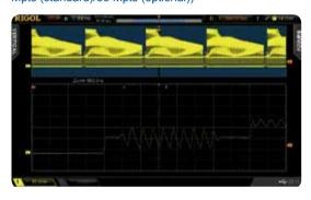
$\label{thm:condition} \mbox{UltraVision: real-time waveform record, playback and analysis functions}$
