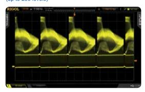
Versatile trigger functions (Runt, Nth Edge, Setup/Hold...)
