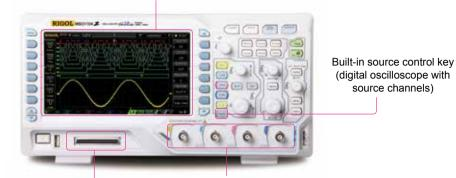
16 digital channels (for MSO1000Z and 4 analog channels MSO upgradable for DS1000Z Plus)
