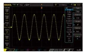
Optional serial bus trigger and decoding functions (RS232/UART, I2C, SPI)
