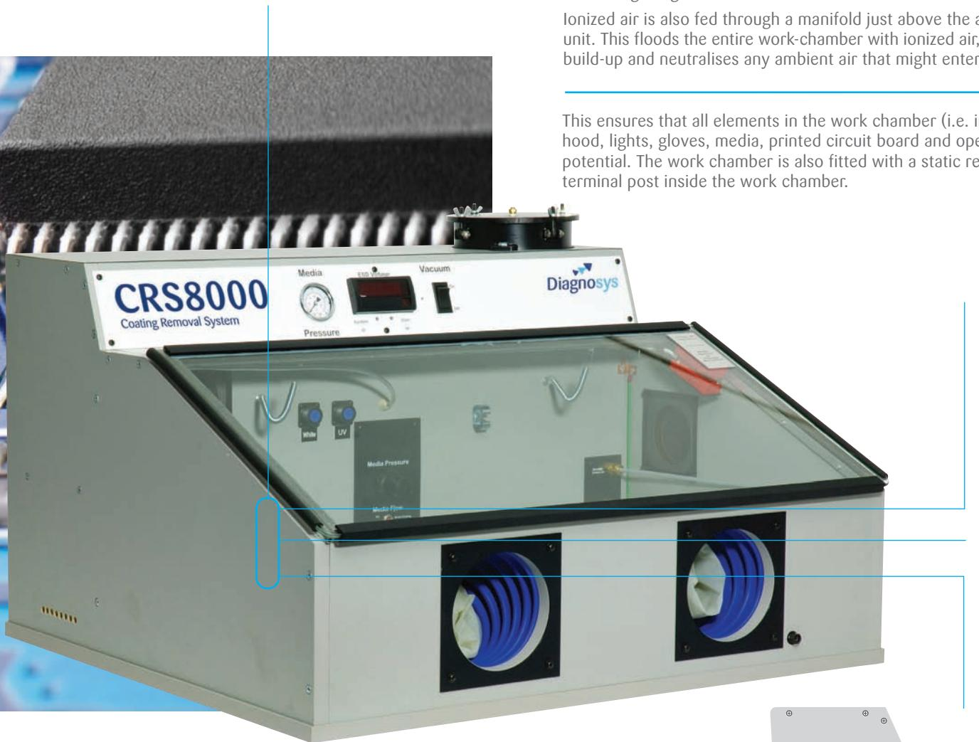
**The Coating Removal System (CRS)** is a self-contained, bench top workstation designed for the safe removal of conformal coatings from printed circuit boards and other electronic devices. It uses a bead blasting technique in a clean and deionised air stream. It is electro-static discharge (ESD) safe and chemical free. The work area is brightly illuminated with both white and UV lights, which are user selectable.
