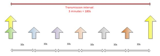
Below diagram shows how TBS12B/TBS12S operate with a 1 hour measurement interval and 3 hours transmission interval:
