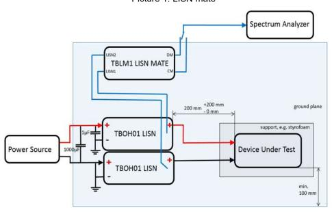
Picture 2: set up for the measurement of differential mode and common mode conducted noise terminate the unused LISN mate output port with 50 Ohm
