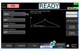
**2** Press Band Pass Filter, and then turn the rotary knob to change the value.
