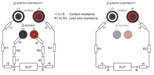
Two-terminal wiring Connect test leads to the OUTPUT LO and HI terminals. The sum of contact resistance r1 to r4, lead wire resistance R1 and R2, and the resistance across A and B is measured.
