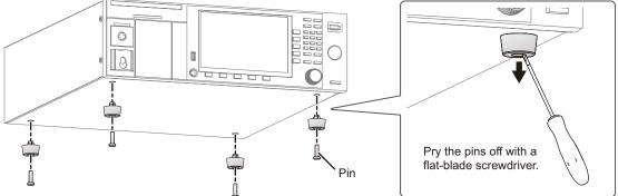
Pry off the pins holding the legs (four locations) with a flat-blade screwdriver.
