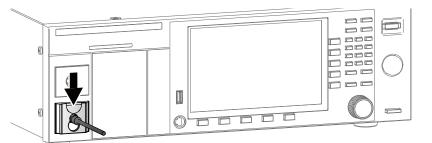
Connect the low-voltage test lead (black) to the EUT.
