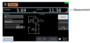
If measuring across terminals A and B (A-B Terminal) is set to VoltMeter (p.205), the DANGER LED lights only when a voltage higher than or equal to the voltage specified by SELV setting (p.206) is present across the terminals A and B.
