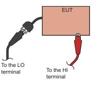
Ex: Between the grounding terminal of the power cord and grounded enclosure
