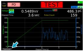
The changed voltage is immediately applied to the test, but the voltage value on the display shows the measured value. When "READY" appears in the upper right of the display after the test is finished, the new voltage setting will be displayed.
