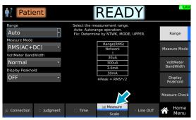
**2** Press Measure Mode and then turn the rotary knob to change the value.
