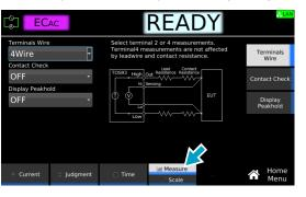
**2** Press Contact Check, and then turn the rotary knob to select ON or OFF.
