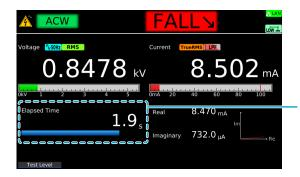
Elapsed time. The remaining fall time is displayed with a bar graph.
