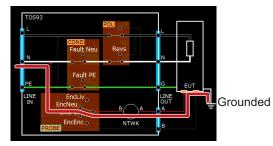
To perform tests safely, it is necessary to check in advance that the measurement point is not grounded. Ground check performs this check automatically. After you press START, a weak current is run between test lead A and the ground to check whether the measurement point is grounded before starting the test.
