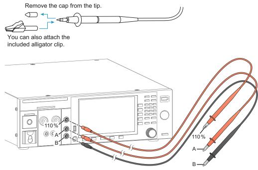
The locations on the EUT that test leads are connected to vary depending on the probe and condition settings of the test conditions and the appliance class of the EUT. For details on touch current testing, see "Connecting the test leads to the EUT" (p.152). For details on patient leakage current testing, see "Connecting the test leads to the EUT" (p.194).
