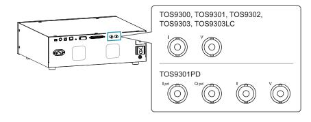
**NOTE** Monitor signal output is isolated from the chassis (earth). If you connect an oscilloscope or an external device whose BNC shield is grounded for other than PD tests, be sure to set the grounding mode (GND) on the test conditions to Guard.
