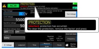
This completes the checking of the interlock operation.
