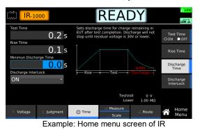
Use the numeric keypad or the rotary knob to enter the time.
