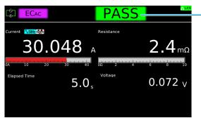
When a test finishes, the judgment result is shown in the test status.
