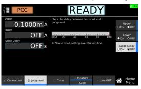
**Press Judge Delay to switch between on and off.** Judge Delay switches between on and off each time you press the key.
