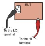
Ex: Between the protective ground terminal and grounded enclosure
