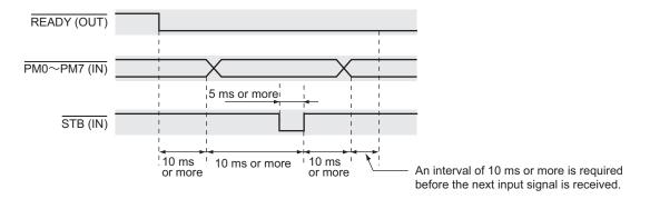
With "READY" shown in the upper right of the display, apply high-level or low-level signals to PM0 (pin 3) to PM7 (pin 10) of the SIGNAL I/O connector.
