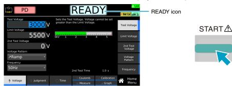
The DANGER LED lights, and the test starts. If the test does not start, see "Unable to start a test" (p.336).
