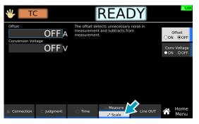
Press Conv Voltage to switch between on and off.
