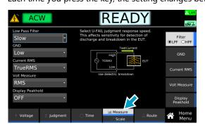
**2** Press Current RMS, and then turn the rotary knob to change the value.
