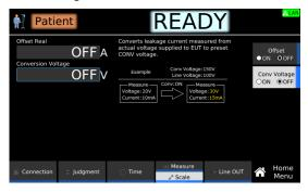
**3** If you select on, use the numeric keypad or the rotary knob to enter the voltage. Setting range: 80.0 V to 300.0 V This completes the setting.
