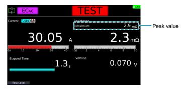
**On the Home menu screen, press Measure repeatedly until Measure is selected.** Each time you press the key, the setting changes between Measure and Scale.
