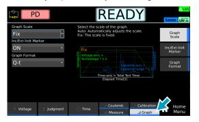
Press Inc/Ext-Volt Marker, and turn the rotary knob to select ON or OFF.
