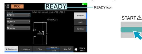
"TEST" is shown in the upper right of the display, and the test starts. If the test does not start, see "Unable to start a test" (p.336).
