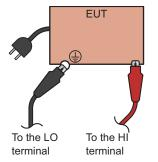
Ex: Between the protective conductor terminal and grounded enclosure
