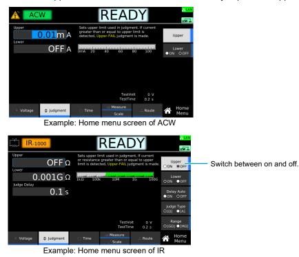
**9** Use the numeric keypad or the rotary knob to enter the current or resistance value.
