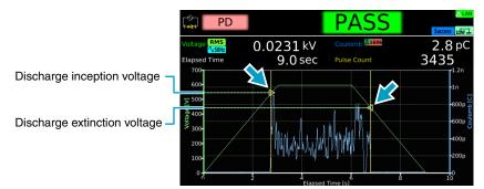
**On the Home Menu screen, press Graph repeatedly until Graph is selected.** Each time you press the key, the setting item switches between Calibration and Graph.
