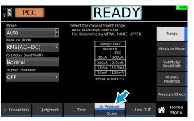
**2** Press Measure Mode and then turn the rotary knob to change the value.
