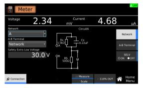
Set the required conditions by referring to the description of measurement conditions (p. 203).
