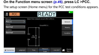
Set the required conditions by referring to the description of test conditions (p.160).
