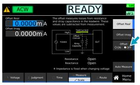
If set to ON, set the Offset Real and Offset imag values according to the following procedure.
