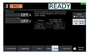
If you select on, use the numeric keypad or the rotary knob to enter the voltage.
