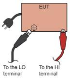
Ex: Between the protective conductor terminal and grounded enclosure
