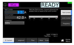
Use the numeric keypad or the rotary knob to enter the current.
