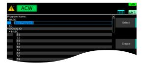
2 Use the numeric keypad or the rotary knob to enter the program name, and then press ENTER.
