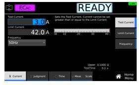
Set the required conditions by referring to the description of test conditions (p.86).
