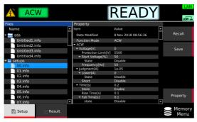
Press Property to view the settings of the setup memory on the right side of the display. Press Property again to return to setup memory selection.
