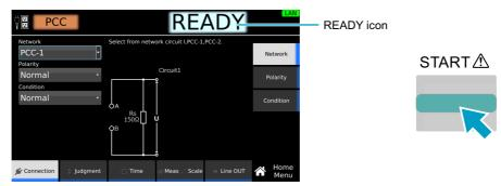
"TEST" is shown in the upper right of the display, and the test starts.
