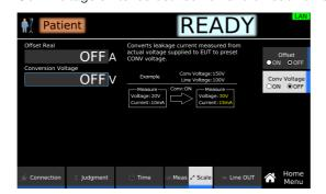
If you select on, use the numeric keypad or the rotary knob to enter the voltage. Setting range: 80.0 V to 300.0 V
