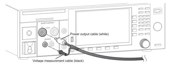
Connect the test lead's current output cable (red) to the EARTH CONTINUITY OUT-PUT HI terminal and the voltage measurement cable (red) to the SENSING HI terminal
