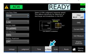
Press Current RMS, and then turn the rotary knob to change the value.
