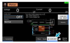
Press 110% OUT to switch between ON and OFF.
