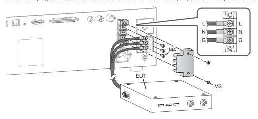
Connect the insulation transformer to the AC LINE IN inlet with the power cord for the EUT.
