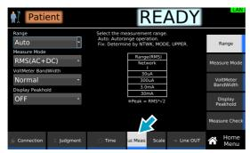
Press VoltMeter BandWidth, and then turn the rotary knob to change the value.
