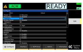
Use the numeric keypad or the rotary knob to enter the duration of time until the product decides that there is no SCPI communication, and then press ENTER.
