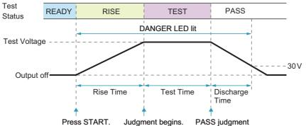
Start Voltage: OFF Upper: ON Lower: ON Delay Auto: ON Test Time: ON Rise Time: ON Discharge Time: 0s
