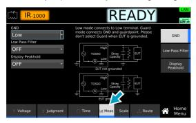
Press Low Pass Filter, and then turn the rotary knob to select ON or OFF.
