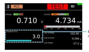
Elapsed time. If Test Time is set to on, the remaining test time is displayed with a bar graph.
