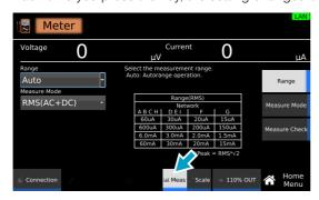
Press Measure Mode, and then turn the rotary knob to change the value.
