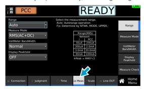
Press Measure Mode and then turn the rotary knob to change the value.
