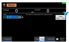
If you select on, use the numeric keypad or the rotary knob to enter the current.
