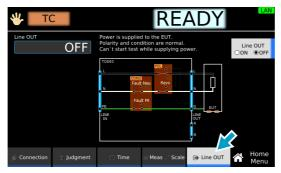
Press Line OUT to switch between on and off.
