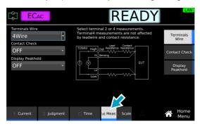
Press Contact Check, and then turn the rotary knob to select ON or OFF.
