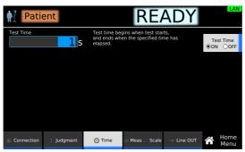
Press Test Time to switch between on and off.
