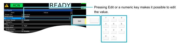
When changing a setting, if there are multiple items you can choose from, select the item using the rotary knob. If there is a number before the item name, you can also select using the numeric keypad. Procedures using the rotary knob are provided in this document.
