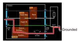
To perform tests safely, it is necessary to check in advance that the measurement point is not grounded.
