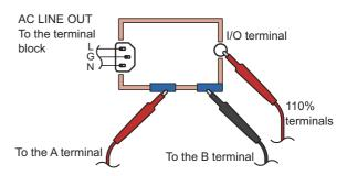
Example 4: Across two points on the enclosure (apply 110% voltage)
