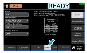
Press Display Peakhold and then turn the rotary knob to select ON or OFF.
