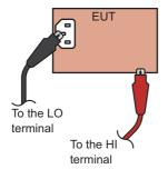
Ex: Between the protective ground terminal and grounded enclosure
