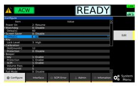
Use the numeric keypad or the rotary knob to set the time until the screen saver is activated, and press ENTER.
