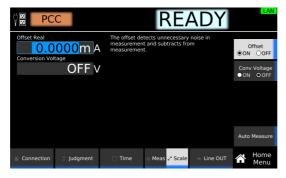
If set to ON, set the Offset value according to the following procedure.
