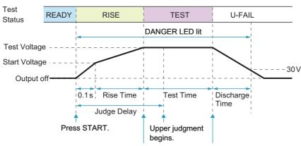
Start Voltage: ON Lower: ON Delay Auto: OFF Test Time: ON Rise Time: ON Fall Time: ON Discharge Time: 10s
