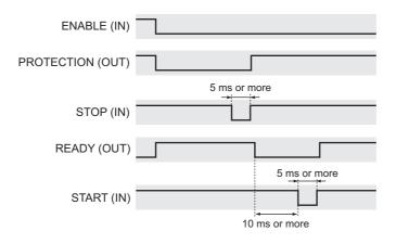
Set ENABLE (pin 17) of the SIGNAL I/O connector to low level.
