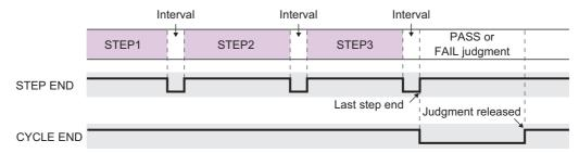
■ If a FAIL judgment is made in the middle of a step and auto test stops
