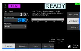
Use the numeric keypad or the rotary knob to enter the current.
