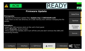
Insert the USB memory device on which the update files have been saved into the USB port on the front panel, and then press Execute.
