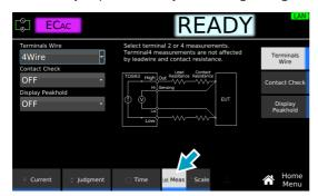
Press Terminals Wire, and then turn the rotary knob to change the value.
