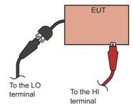
Ex: Between the grounding terminal of the power cord and grounded enclosure
