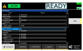
Use the rotary knob or numeric keys to enter the calibration period, and then press ENTER.
