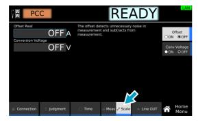
Press Offset to switch between on and off.
