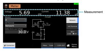
If Measuring across terminals A and B (A-B Terminal) (p.173) is set to VoltMeter and voltage exceeding the value set with SELV setting (p.174) is present across terminals A and B, the DANGER LED lights.
