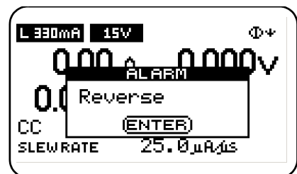
Fig. 2-11 Reverse connection alarm
