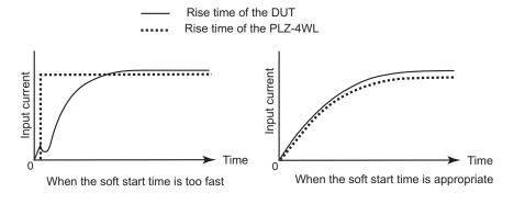
If the current rise time that is determined by the slew rate and the current setting is longer than the soft start time, the actual rise time will be longer than the soft start time. If you want to raise the current according to the soft start time, increase the slew rate.
