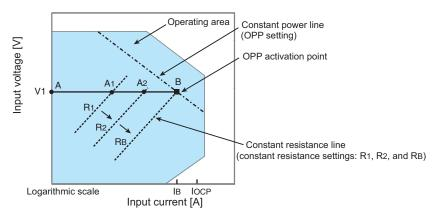
If the overcurrent protection (OCP) setting IOCP is greater than the current value IB at point B, when the PLZ-4WL resistance is decreased (R1 $\rightarrow$ R2 $\rightarrow$ RB) so that the input current (load current) increases, with the voltage of the constant-voltage power supply at V1, the operating point moves along segment AB (A1 $\rightarrow$ A2 $\rightarrow$ B). When point B is reached, overpower protection (OPP) is activated.
