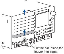
Attach the louver so that its tabs enter the slots in the panel. While pushing on the second slat from the bottom of the louver, slide the louver up to attach it to the PLZ-4WL.
