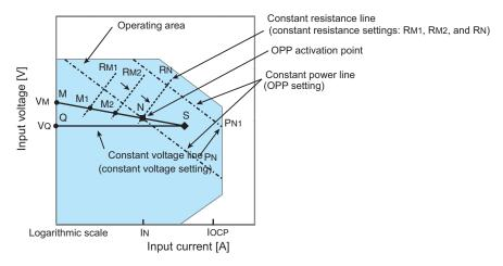
When the overcurrent protection (OCP) setting IOCP is greater than current IN at point N, the voltage of the battery is VM. In constant resistance (CR) mode, if the resistance is reduced (RM1 $\rightarrow$ RM2 $\rightarrow$ RN) so that the input current (load current) increases, the operating point moves along segment MN (M1 $\rightarrow$ M2 $\rightarrow$ N).
