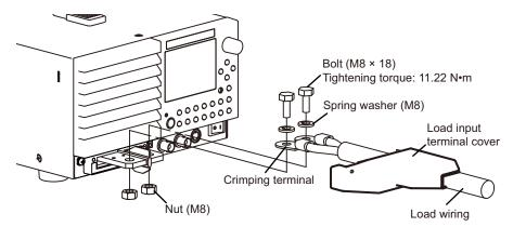
Using the PLZ-4WL's screws, connect one end of the chassisconnection wire that came with the PLZ-4WL to the chassis, and connect the other end to the negative load input terminal.
