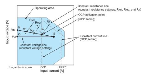
When the overcurrent protection (OCP) setting IOCP is lower than the current produced by the activation of overpower protection (OPP), the voltage of the battery is VM. In constant resistance (CR) mode, if the resistance is decreased (RM1 $\rightarrow$ RM2 $\rightarrow$ RT) so that the input current (load current) increases, the operating point moves along segment MT (M1 $\rightarrow$ M2 $\rightarrow$ T).
