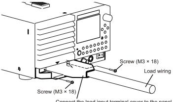
Connect the load input terminal cover to the panel so that the terminals are not exposed.
