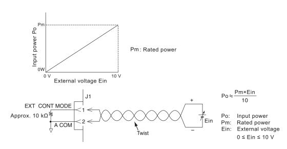
To avoid noise interference, use a highly stable, low-noise external voltage source and twisted signal wires.
