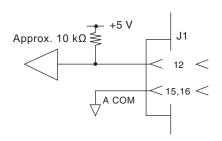
Apply an external signal to pins 12 and 15 or 12 and 16 of the J1 connector.
