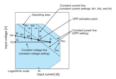
The battery voltage is VM. In constant current (CC) mode, if the current is increased ( $IM1 \rightarrow IM2 \rightarrow IN$ ) so that the input current (load current) increases, the operating point moves along segment MN ( $M1 \rightarrow M2 \rightarrow N$ ).
