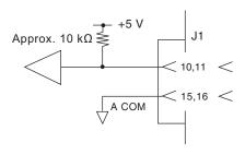
Use pins 10 (RANGE CONT 1) and 11 (RANGE CONT 0) of the J1 connector (use pin 15 or 16 as the common).
