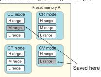
In CC+CV mode, memory entries for CC mode and CV mode are used. In CR+CV mode, memory entries for CR mode and CV mode are used.
