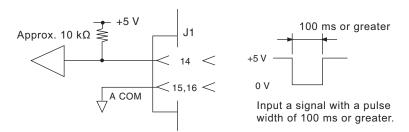
After an alarm has occurred, a low level signal applied after the reason for the alarm has been eliminated releases the alarm.
