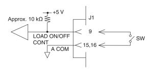
The input pin is pulled up to the internal circuit's +5 V level by a resistor that is approximately 10 k $\Omega$ . The maximum allowable voltage is 5 V. The logic threshold levels are CMOS.
