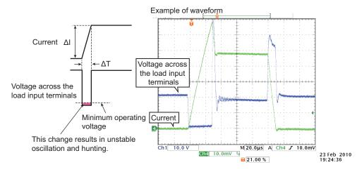
To make sure that the voltage resulting from inductance remains within the range of the electronic load's minimum operating voltage and maximum input voltage, make the wiring as short as possible and twist the wiring, or reduce the slew rate. If it is not necessary to operate at a high response speed, reduce the slew rate in CC mode, or reduce the response speed in CR mode.
