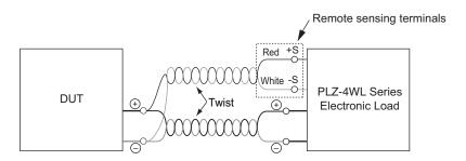
The table below indicates sizes of the wires that you can use to connect to the sensing terminals. Strip approximately 10 mm of coating from the end of the wiring.
