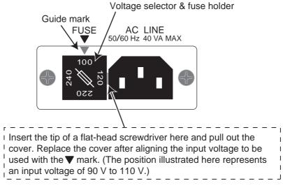
Fig. 1-2 Removing the fuse holder
