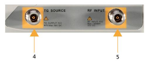
Figure 1-9 Front Panel Connectors
