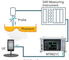
**SAR Test Setup**
